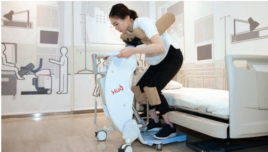
The robot Hug is designed to assist care workers in lifting people, a demanding physical job.
