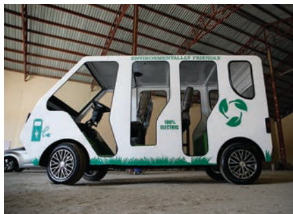
Phoenix Renewables maintains a fleet of a dozen retrofitted electric minibuses capable of covering a distance of 150 kilometers on a charge.
