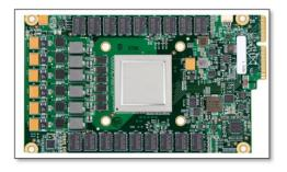
TPUs were purpose-built specifically for AI. TPUs are an application-specific integrated circuit (ASIC), a chip designed for a single, specific purpose: running the unique matrix and vector-based mathematics that's needed for building and running AI models.
