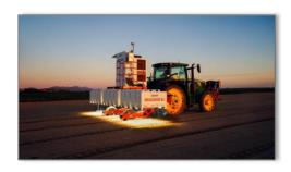
The LaserWeeder leverages our sophisticated laserweeding technology, driven by AI deep learning models and computer vision software, to efficiently identify, target, and eliminate weeds by zapping them at the meristem. The implement can cover up to 2 acres per hour and shoot up to 200,000 weeds.
